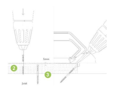
For best results, coat the fixings in silicone spray before use. When screwing in, push firmly on the screw whilst applying pressure to the board (2), finishing the screw head 5mm below the Lastane<sup>®</sup> surface. This should leave a minimal witness mark (3).
